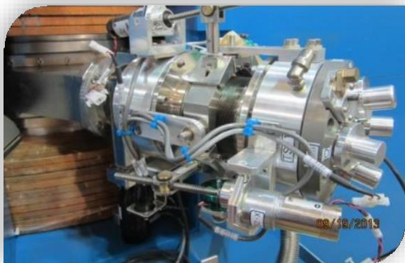
Multi-port target selector (up to 150 \mu A of beam current)
