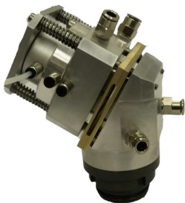
30° solid target holder for solid target
